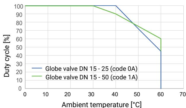
Control module positioner (code S0, S5, S6), control operation - class C acc. to EN 15714-2
