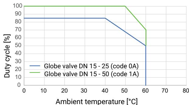
Control module Positioner (code S0, S5, S6), Open/Close duty
