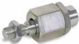
Flexo coupling for articulated mounting of piston rod. Flexo fitting is intended to take up axial angle errors within a range of  $\pm 4^\circ$ .
