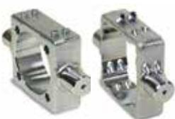
Available for P1F Profile and Tie-Rods versions the MT4 centre trunnion when combined with AT4 pivot brackets is intended for articulated mounting of the cylinder. The trunnion is free so that it can be fixed afterward when the cylinder is at the right place on the machine.
