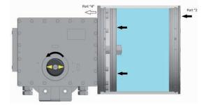
Air supplied to port 4 forces the piston far from the central module/toward the end of the power module. A clockwise rotation is achieved. Exhaust air flows from the port 2
